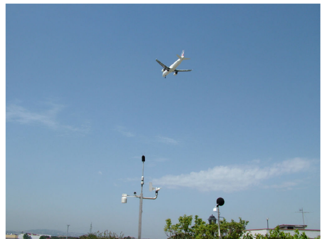
Fig. 10 A320 landing noise measurement.
